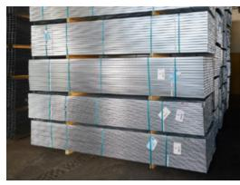
The products are manufactured from hot dip galvanized carbon steel. Purchased galvanized coils are divide into narrower bands whose width fits the specific profiles and accessories. Then, steel profiles are manufactured through roll forming technique while accessories are cut from bands according to relevant specifications.
