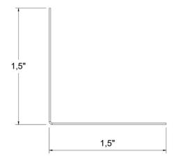
Web Depth 1,50 in Flange Width 1,50 in **Design Thickness** 0,0188 in Minimum Thickness 0,0179 in Yield Strength: 33 ksi Cross Sectional Area 0,056 in2 Unit Weight Finish G40
